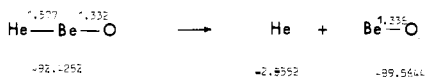
Chart II. Calculated Energies [hartrees] and Bond Distances [Å] for HeBeO and BeO at the CASSCF Level
